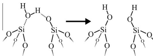
**Fig. 4.** Adsorption–dissociation reaction mechanism between H<sub>2</sub>O and a ruptured bridge.
