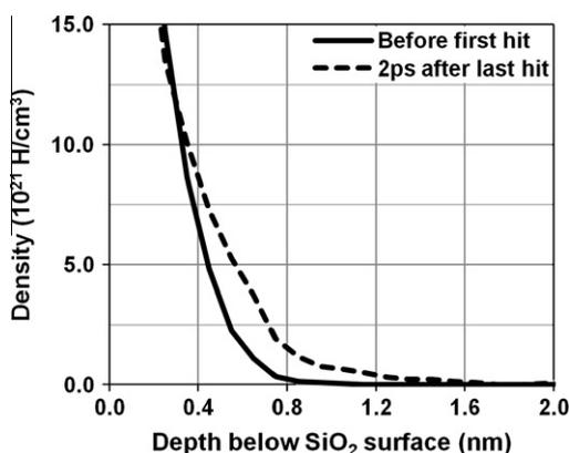
Fig. 6. Density of hydrogen in the silica subsurface.
