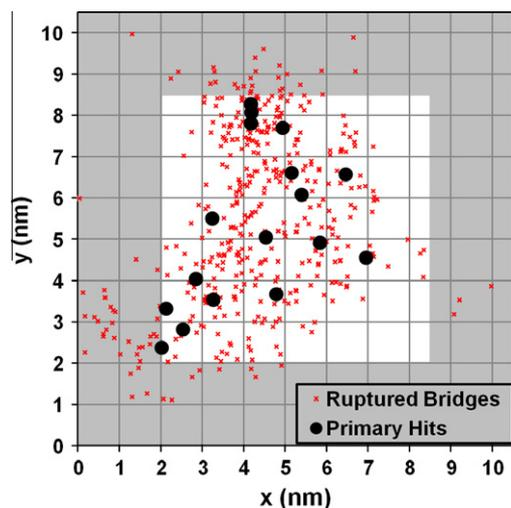
**Fig. 3.** Distribution of PKAs and consequent net damage in the  $x$ - $y$  plane. All PKAs were chosen randomly from the non-shaded region. Ruptured bridges shown reflect the positions of bridges that ruptured following a decay event and did not re-form into a bridging site during the 2 ps following that decay.
