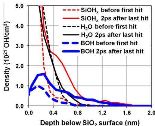
Fig. 7. Density and coordination of H as a function of distance into the silica subsurface before and after radiation damage.
