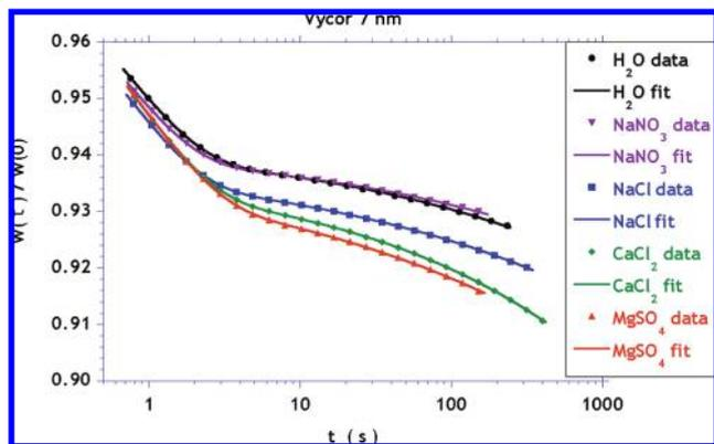
**Figure 1.** Relaxation of load,  $W(t)$ , measured on 7 nm Vycor rods containing pure water or 1 M solutions of various salts.
