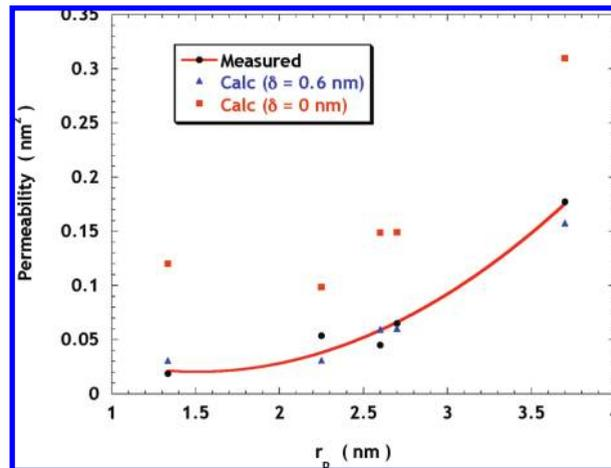
**Figure 4.** Permeability measured in porous glasses with various pore radii,  $r_p$ . Circles are measured values, and triangles are calculated from the Carman–Kozeny equation assuming that the thickness of the immobile layer is  $\delta = 0$  ( $\Delta$ ) or 0.6 ( $\blacktriangle$ ) nm.
