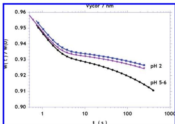
**Figure 2.** Relaxation of load,  $W(t)$ , measured on 7 nm Vycor rods containing 1 M solutions of  $\text{CaCl}_2$  with the pH adjusted to 2 (upper two curves) or not.
