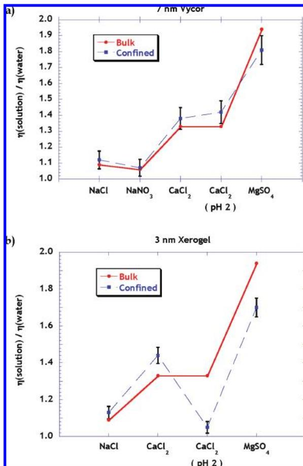
**Figure 5.** Ratio of viscosity of 1 M solutions to that of water for bulk solutions and for liquids confined in (a) 7 nm Vycor or (b) 3 nm Xerogel. Error bars are standard deviations based on a range of measured values.
