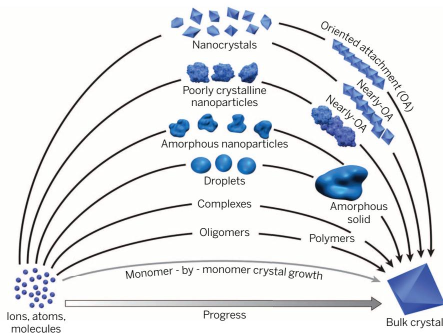
**Fig. 1. Pathways to crystallization by particle attachment.** In contrast to monomer-by-monomer addition as envisioned in classical models of crystal growth (gray curve), CPA occurs by the addition of higher-order species ranging from multi-ion complexes to fully formed nanocrystals. (The final faceted bulk crystal is a schematic representation of a final single-crystal state. As Figs. 2 and 3 show, the final crystal can have more complex morphologies, including spheroidal.)
