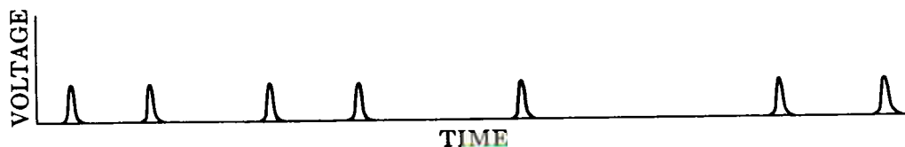
Fig. 7-9 Randomly spaced voltage pulses produced by a counter.
